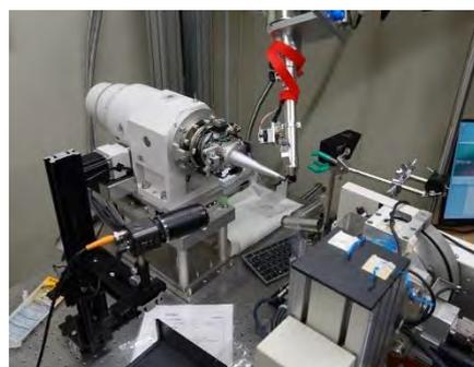
Fig. 4. Laser irradiation and crystal freezing system for cold trapping of intermediate states
